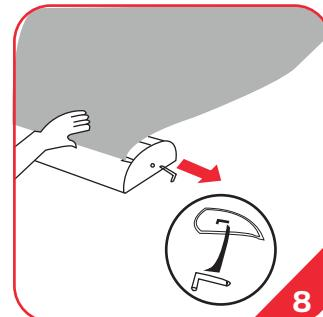
8.Peel off the cover, remove the screw underneath the chrome end of the base and detach. Then, with the graphic held firmly, carefully pull out the retaining pin, then put it into the cover.
