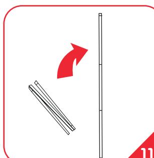
11.Unfold the pole and slip the pieces together to assemble it to a rigid pole(the hooked end corresponds to the top and the round end belongs to the bottom base).
