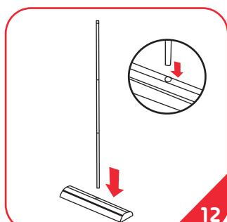
12.The bottom of the assemble pole slides into the round socket in the centre of the base unit.
