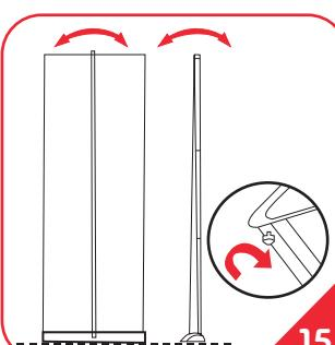
15.The unit can be levelled by adjusting the threaded feet at the bottom of the base unit.
